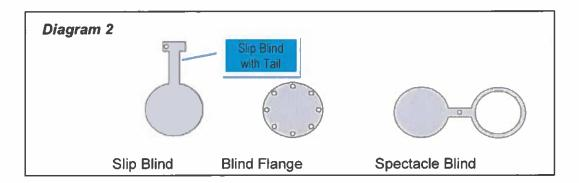
The rating, size and location of all blinds shall be verified prior to installation and shall be reflected on the blind list. Each blind shall be stamped with the corresponding pressure rating and installed with matching gaskets. Temporary blinds shall be of a specific color to be easily identified.
