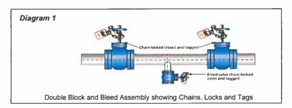
Single block valve and DB&B isolations shall not be used when equipment or a piping containing hazardous materials is to be opened for confined space entry or hot work activities. Both activities require isolation by blinding or isolation.
