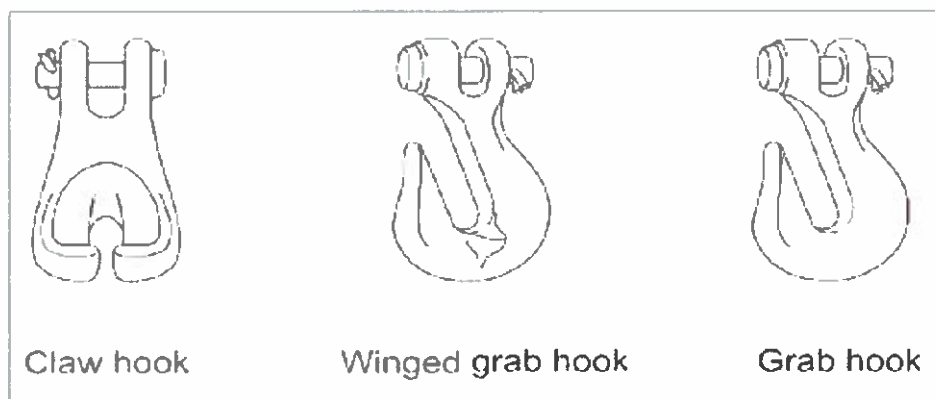
Figure 2 – Chain Hook Type
